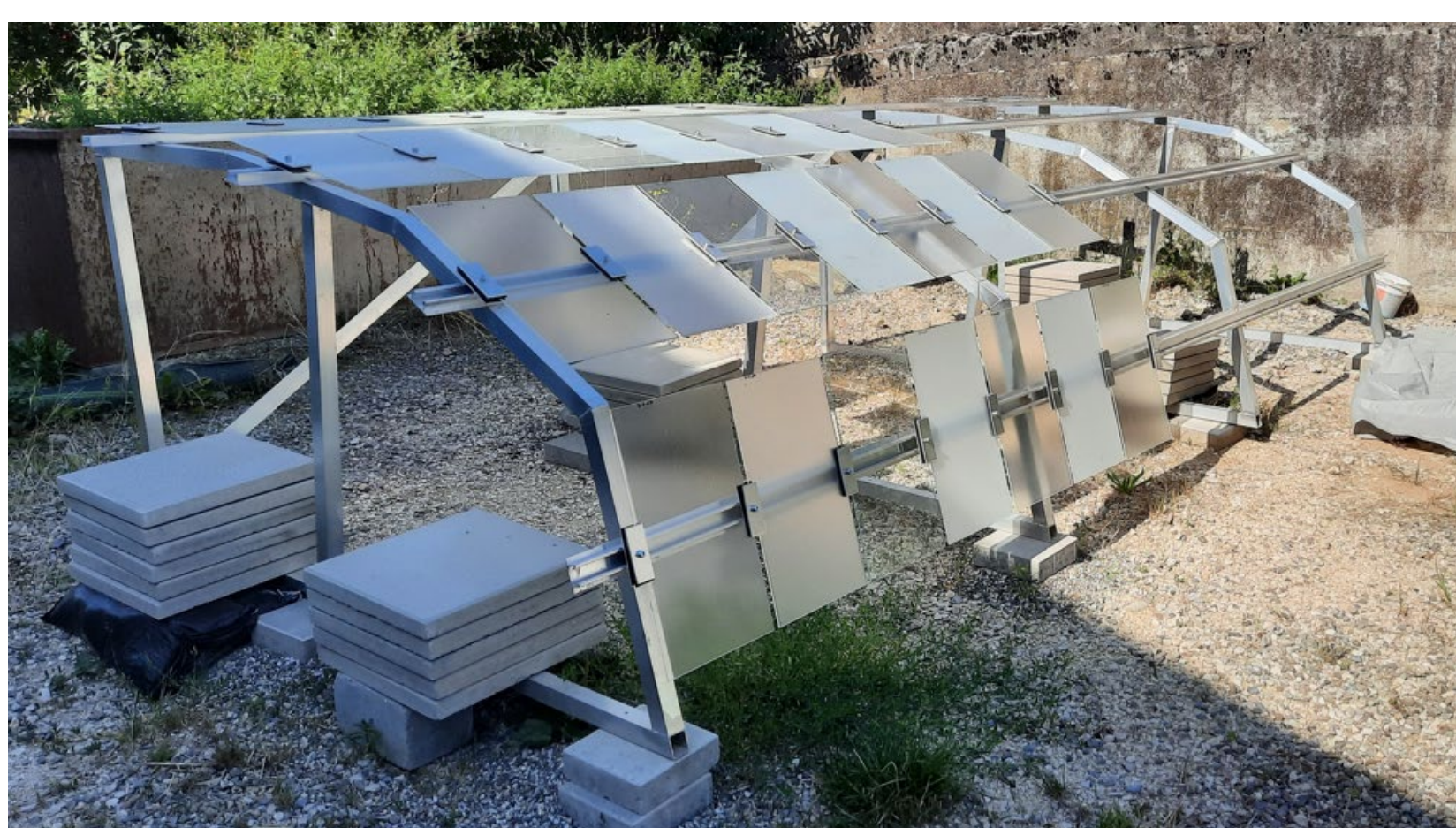
Figure 2: First prototype of the soiling test bench
